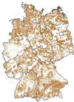
Figure 6-1: Eligible land (colored areas) for onshore wind generation in Germany according to the scenario assumptions [24].
